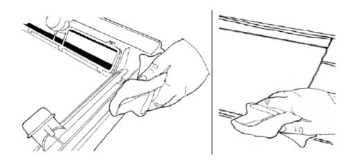
**Step 5:-** Apply a continuous bead of **Non Acetic** silicone a minimum of 6mm wide to the centre of the flange all the way around the hatch. **Do not over apply.**
